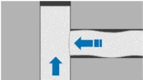
Note especially for the window assembly when cutting of the tape: the addition of at least 1 cm per meter of joint length.
