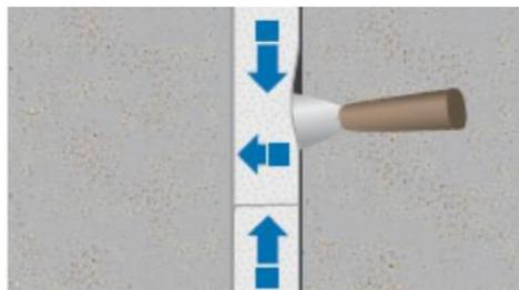
At vertical joints start at the bottom and continue working upwards. Press the adhesive side (possibly with a spatula) firmly against the joint edges. The joints of abutted tapes must be compressed against each other, but take care not to stretch the tape.
